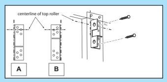
FIG. 2-8 Examples of door bracket positioning.
